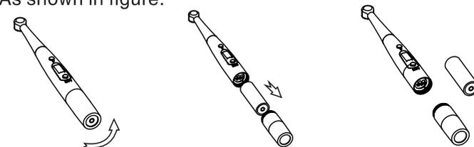
4.2 Press and install the shading sheet on the light guide head.
